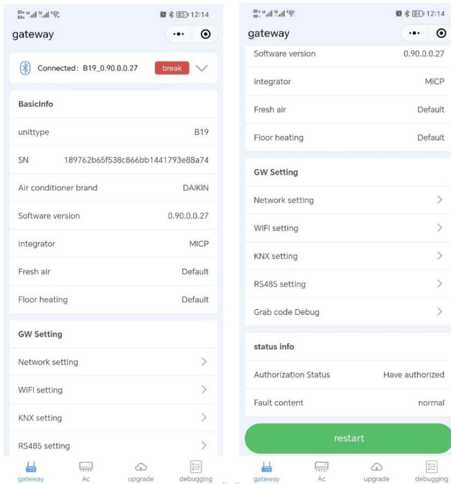
Basic information: including equipment model, SN code, controlled air conditioner brand, product software version, integrator information, controlled fresh air, controlled floor heating.
