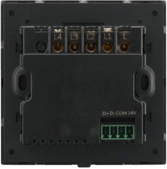
Panel power interface with 4CH relay
